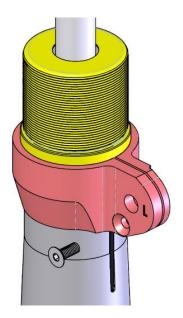
13. Install the spring perch and black plastic isolator disc (in Coil-Over Hardware Kit) as shown. Adjust the perch to about 3/8" up from bottom. This will be the starting ride height setting, and should get you close to Dinan's target ride height. Snug the 6mm screw to lock the perch into place.
