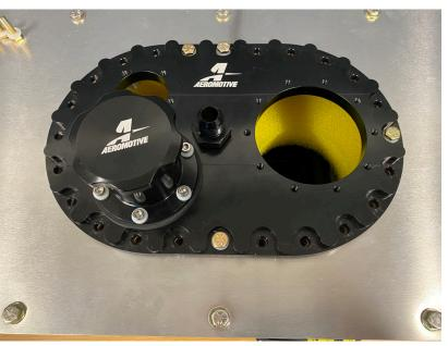
Line up the holes of the cell, gaskets, top plate, and nut ring and install a few pieces of hardware.
