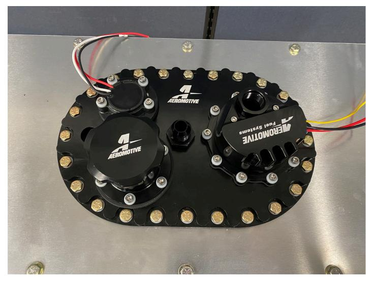
Note: Vent rollover valve is missing from the above assembly.
