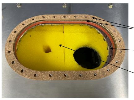
Elements that should be in place before top plate is installed.
