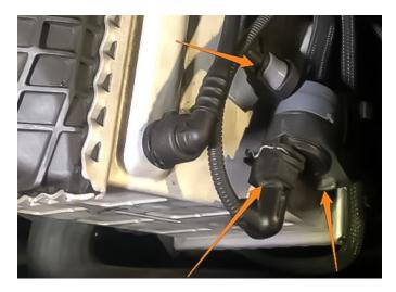
**08.** Remove the MAP sensor electrical connector and loosen the clamp connecting the throttle body coupler to the intake manifold, on the throttle body side. Repeat on other intercooler.
