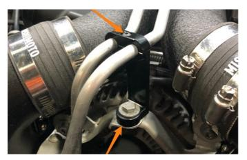
23. Vacuum fill the intercooler cooling system and check for leaks and make sure that all electrical connections are connected.
