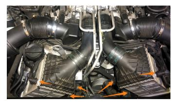
**07.** Remove the EVAP electrical connector, EVAP line, and remove the EVAP solenoid from the EVAP bracket from each intercooler. (Image on right)
