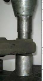
When pressing out bushings, it is good practice to remove and replace one at a time to maintain good rear alignment.
