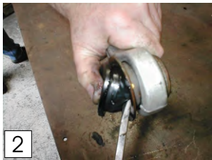
Remove OEM rubber.
