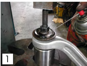
Remove inner sleeve.
