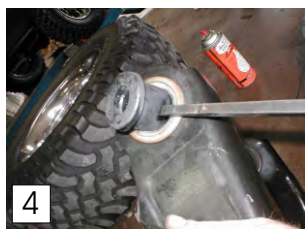
Remove OEM rubber.
