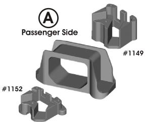
**NOTE:** Must cut the ties and buttons to relieve the shaded portions depicted in the figure to the right. This allows them to clear the casting without inhibiting the inherent movement of the motor mount. **REMEMBER:** Do not overtighten the ties or they will break when the motor torques.
