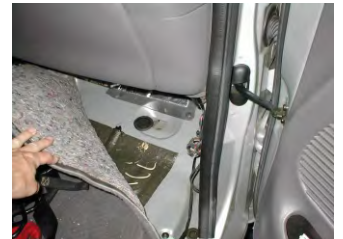
Lift carpet in passenger area.
