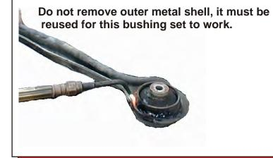
Apply light heat evenly around the outside of the outer metal shell, just enough to brake the bond with the rubber. When you see light smoke coming from the sides of the bushing the bond should be broken. At no time should there be any flames coming from the rubber, if there are any flames, you need to back off with the heat. Just push the old rubber and inner metal sleeve out. Let the outer metal shell cool before cleaning the inside.
