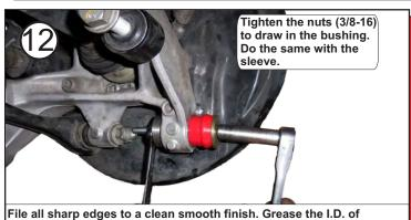
knuckle, I.D. & O.D. of bushing 03P03606 and O.D. of sleeve 15.10.335.39. Using some althread, nuts and flat washers, press in bushing 03P03606 first, then press in the inner metal sleeve
