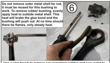
Use a wire brush to remove any remaining rubber and pray paint to prevent rust.
