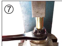
Grease the I.D. of tie rod, I.D. & O.D. of bushing 03P03604 and O.D. of sleeve 15.10.472.39 (inner position) and 03P03603 and sleeve 15.10.419.39 (outer position). Press in bushing 03P03604 or 03P03603 first, then press in the inner metal sleeve 15P1071539 and 15.10.419.39.
