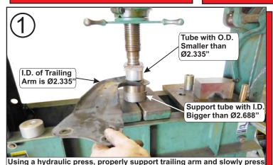
out the rubber bushing with bonded outer metal casing.
