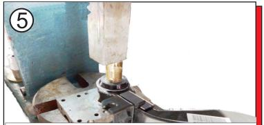
Grease the I.D. of track arm, I.D. & O.D. of bushing 03P03605 and O.D. of sleeve 15P1071639 (inner position) and sleeve 15.10.419.39 (outer position). Press in bushing 03P03605 first, then press in the inner metal sleeve 15P1071539 and 15.10.419.39.
