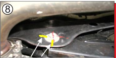
Before removing the lower transverse link, place matchmarks on the front and rear of the adjusting cam bolts. You will need to use these matchmarks to reinstall the transverse link back in the same position after the new polyurethane bushings are installed.
