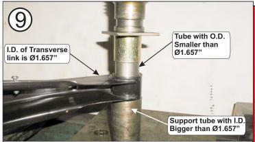
Using a hydraulic press, properly support transverse link and slowly press out the rubber bushing with bonded outer metal shell.
