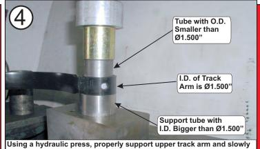
press out the rubber bushings with bonded outer metal casing from both ends of the track arm. The eyes are the same size.
