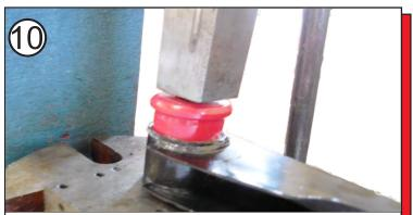
Grease the I.D. of transverse link, I.D. & O.D. of bushing 03P03602 and O.D. of sleeve 15.10.472.39. Press in bushing 03P03602 first, then press in the inner metal sleeve 15.10.472.39.
