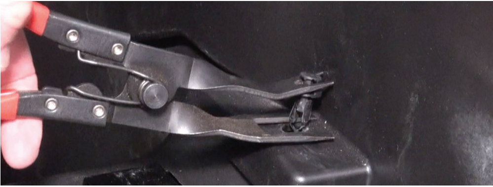
Fig. 3 - Remove push pins from entire perimeter of center console. You can use tool as shown or a flat head screw driver to pop up the center of the push pin, then pull it out of the hole
