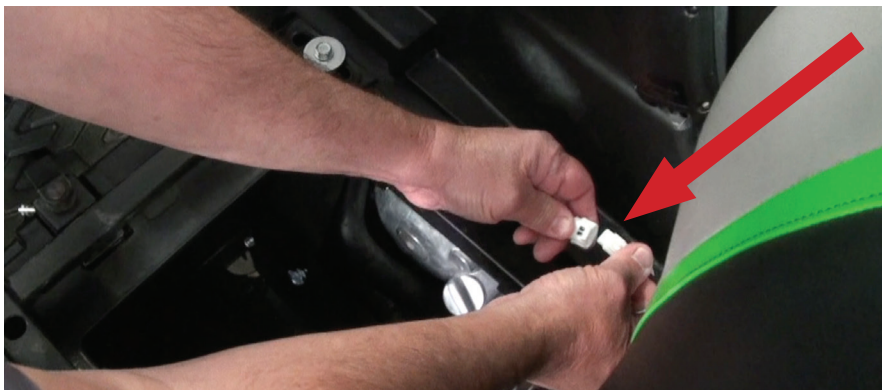
Fig. 1 - Remove driver seat bottom and disconnect seat belt warning connector
