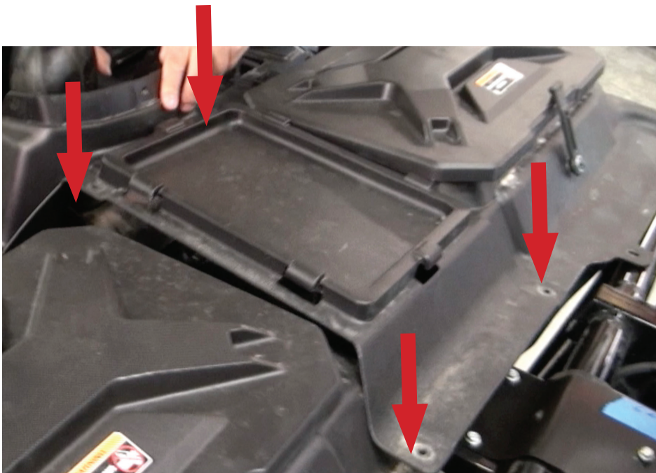
Fig. 7 - Remove 4 screws from center panel between rear storage units & lift panel out
