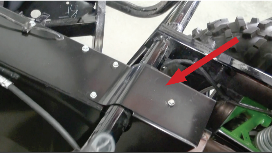
Fig 15 - Remove the top shield on the rear top of the exhaust tunnel.
