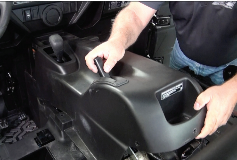
Fig. 4 - After removing all push pins, even the ones in the foot well area, pull up on the back of the console, then lift up and toward the rear of the vehicle to help in removal. Also, engage the parking brake to help in removing the console. This will take some patience.
