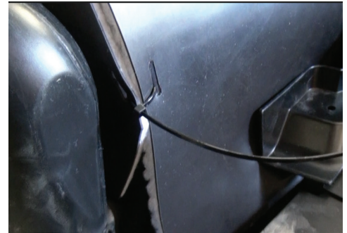
Fig 23 - Secure rear through slots with zip tie
