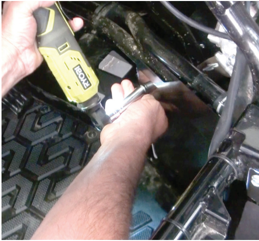
Fig 12. Remove metal heat shield in the drivers foot well
