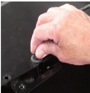
Fig 17 - Oxygen Sensor wire comes through top of panel. Slide grommet and wire out of this panel.
