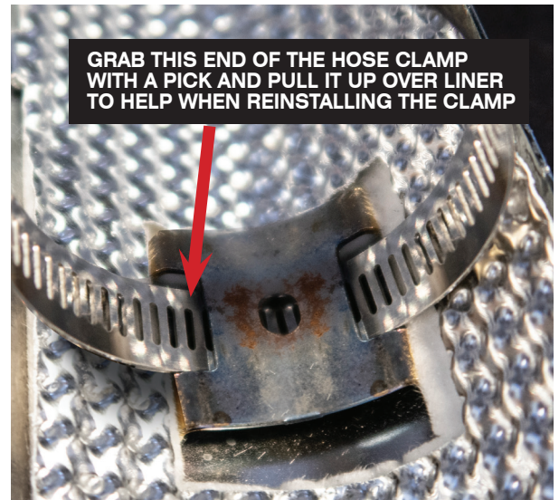
FIG. 6 A PICK WILL HELP REINSTALLING THE CLAMP BY GRABBING IT AFTER IT IS PUSHED THROUGH THE WELDED ON BRACKET AND PULLING IT UP OVER THE LINER.
