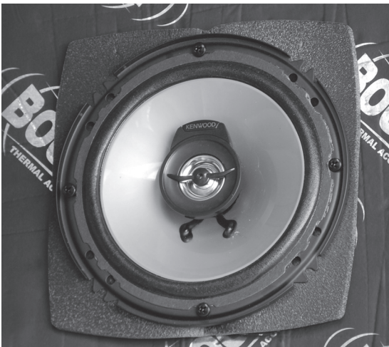
Fig 5 - Secure the speaker & baffle in place with original mounting screws
