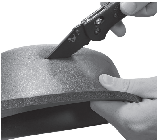
Fig 6 - If bass response is affected by baffle, cut a hole in the bottom side of the baffle to allow air flow for bass.
