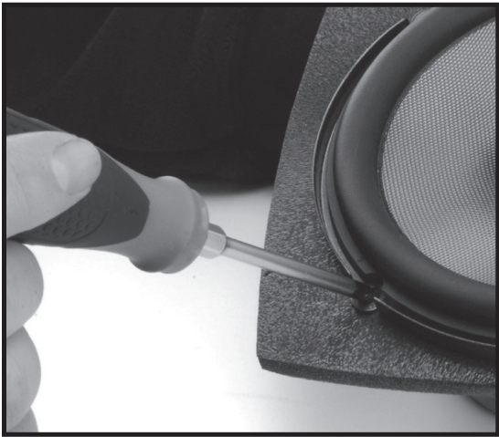
Fig 4 - Make small holes for mounting screws
