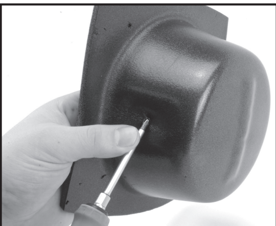
Fig 2 - Make small hole to run speaker wire through
