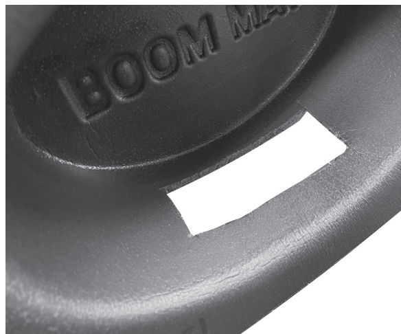
Fig 7 - Cut hole in the side of the baffle that will be facing down when it is installed.
