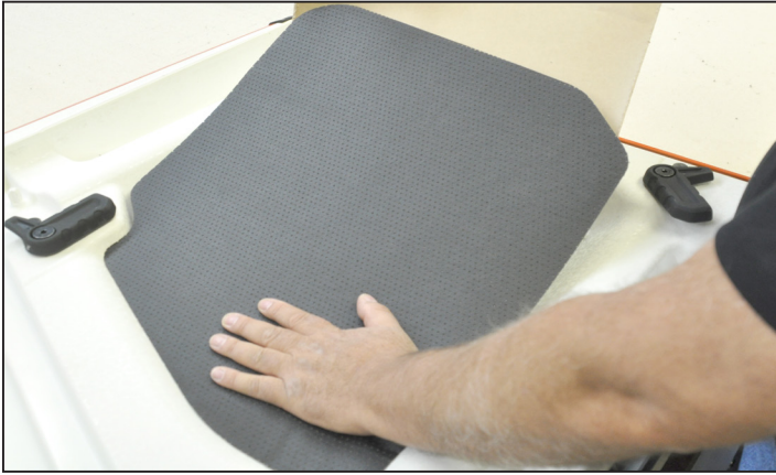
Figure 5. Lay panel in place by applying gentle pressure
