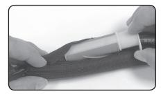
Hold the ends of the lines/wires and the line sleeving and begin to pull the tool away from the starting point.
