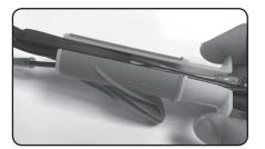
Twist the white part of the tool until the openings in the orange section and white section line up. Insert your wires/cables then twist closed.
