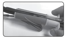
Twist the white part of the tool until the openings in the orange section and white section line up. Insert your wires/cables then twist closed.
