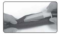
Hold the ends of the lines/wires and the line sleeving and begin to pull the tool away from the starting point.
