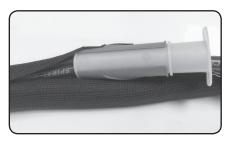
The tool will open up the line sleeving and insert the wires while pulling the tool along the sleeving.
