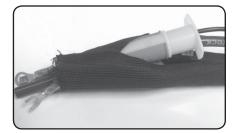
Insert the bottom "spike" of the tool into the line sleeve with the wires and lines sticking out the front of the tool and line sleeving.
