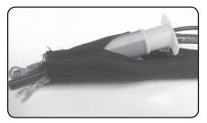
Insert the bottom "spike" of the tool into the line sleeve with the wires and lines sticking out the front of the tool and line sleeving.
