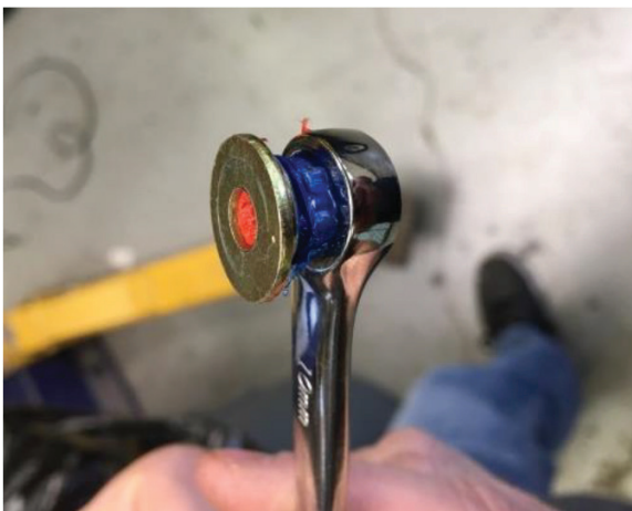
FIG 3. to reinstall side netting anchor, place some tape around the nut and silicone on the washer in order to keep it stationary in the wrench.
