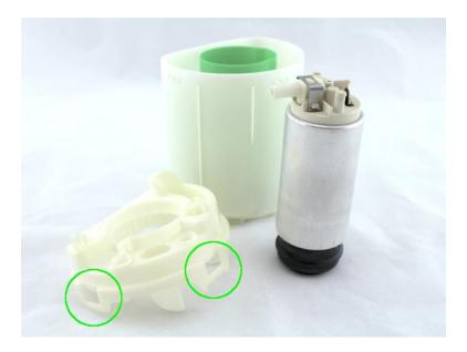
5 – install the 3 supplied o-rings on the DW65v, use a generous amount of Super Lube for smooth installation
