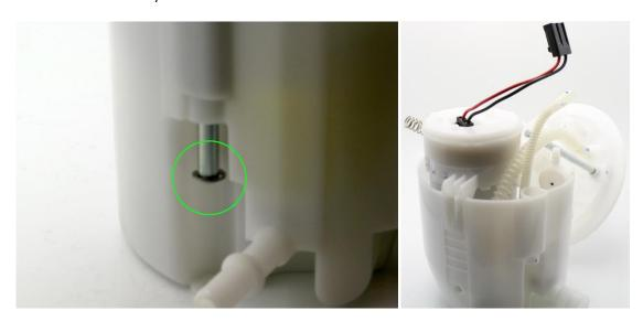
4 – remove the center section from the bucket by lifting the 3 tabs (circled in green)
