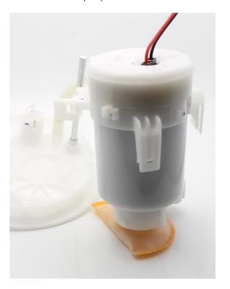
8 – install the center section back into the bucket
