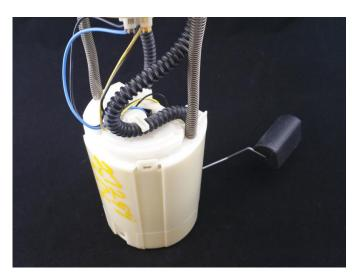
8 – reinstall the assembly into the fuel tank and attach a length of hose to the outlet of the pump assembly allowing it to drain into a fuel safe container and prime the fuel pump assembly
