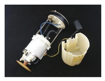
2 – separate the pump cap from the center section of the assembly by lifting the two (x2, green circled) tabs and pulling the cap to the side. Disconnect the electrical connector with a regular screwdriver and then pull the pump out by pulling down
