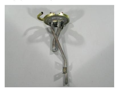
2 – the DW65c/300c has a preinstalled hose and clamp on the pump outlet. Slip the hose clamp over the pre-installed hose. Install the DW65c/300c onto the assembly and tighten the hose clamp
