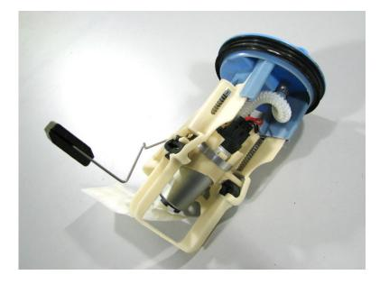
5 – adjust the height of the pump in the pump holder until the pre-filter is near the bottom of the assembly, and tighten the large hose clamp. Do Not Overtighten – pump damage can occur.
