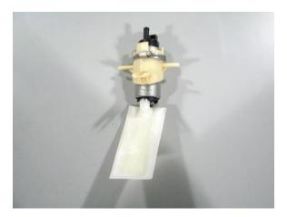
4 – wire in the supplied electrical connector (red-to-red and black-to-brown) and push the PTFE hose onto the assembly inlet. Secure the pump in place using the OE rubber isolators
