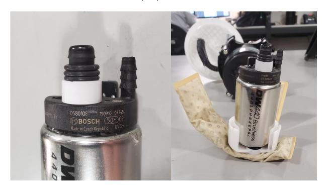
6 – Install the pump into the center section, all 3 of the O-rings should be seated inside the inlet of the module center section, lock the pump into place by latching the three lock tabs on the filter sock retainer.
