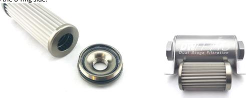
3 – the cap with the spring is the INFLOW! The magnet should be readily visible on the filter element and the smaller diameter of the spring presses into the dish of the filter.
