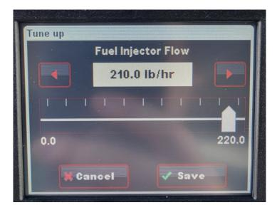
4. After the flowrate has been input the vehicle will need to be driven to relearn each condition as the injector characteristic will have changed. This should allow for the vehicle to be started and driven in low load conditions until the ecu has fully relearned.
