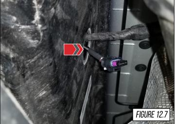
Routing the harness to the valved H-Pipe (part B59) must be done thoughtfully, keep clear of moving components like the driveshaft, and that sweet new exhaust system.
