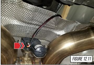
Once the harness is connected to the valve motor at the H-pipe, any slack in the harness needs to be secured to minimize any potential movement.
