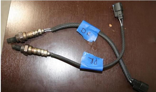
3. Remove the rear O2 sensors and label their positions using a 22mm wrench or O2 sensor socket and 3/8" ratchet. **PRO TIP:** Label on the connector or the sensor body itself. **EXAMPLE:** DR for Driver Rear. PR for Passenger Rear.
