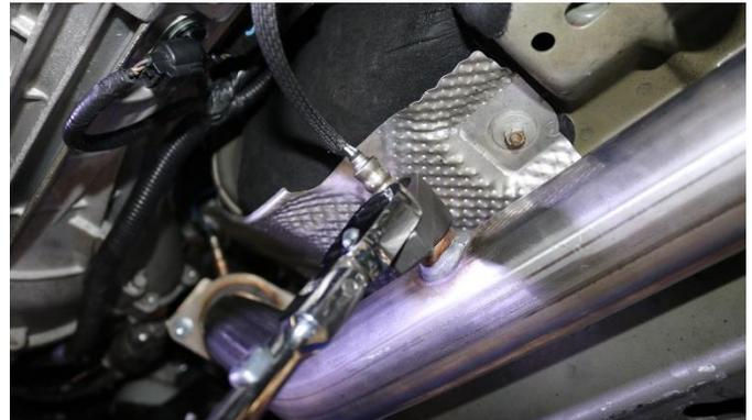
**8.** Install both driver and passenger oxygen sensors onto the off road pipes as shown, tighten with a 22mm O2 sensor socket or wrench.
