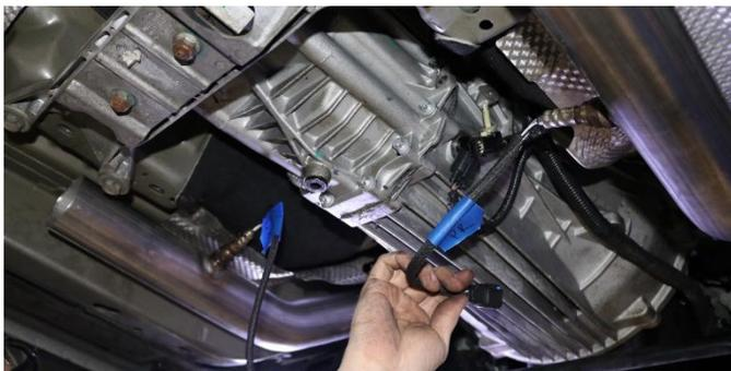
**9.** Plug O2 sensors into off road pipes as shown in picture.
