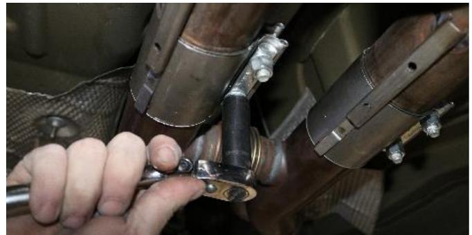
6. Using a 15MM socket or wrench, loosen the factory sleeve clamps (4 Bolts) after the H-Pipe assembly.
