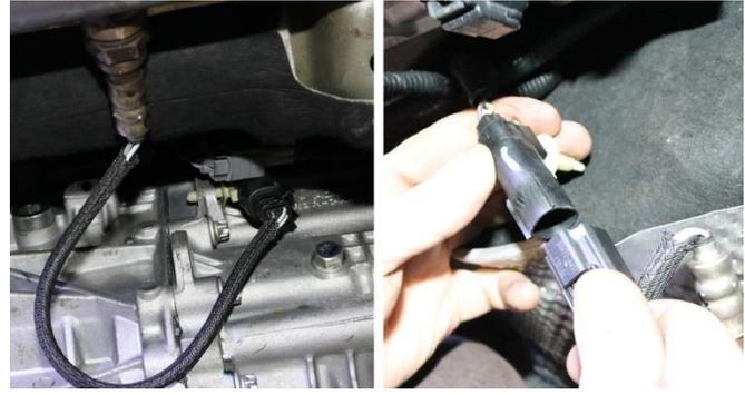
2. **Lift the vehicle and safely secure it.** Disconnect the driver and passenger rear O2 sensor connectors. **PRO TIP:** Disconnect the rear sensor connector from its mount in the transmission to remove it.
