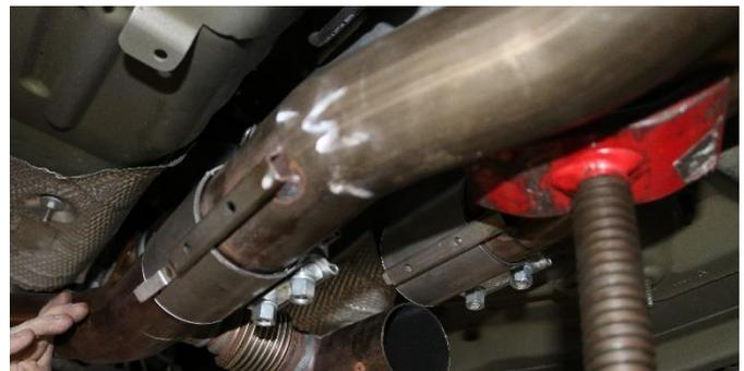
**10.** You may need another person to help support the X-Pipe and keep it from drooping, so the exhaust does not damage the tip cutouts in the factory rear valance.
