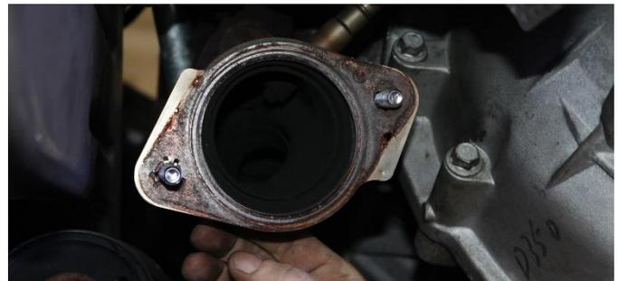
2. Locate the mounting hardware and the two gaskets from **Removal Step 12**. On the driver side, insert the two supplied bolts through the stock manifold flange from the top. Insert the gasket onto the bolts as show.
