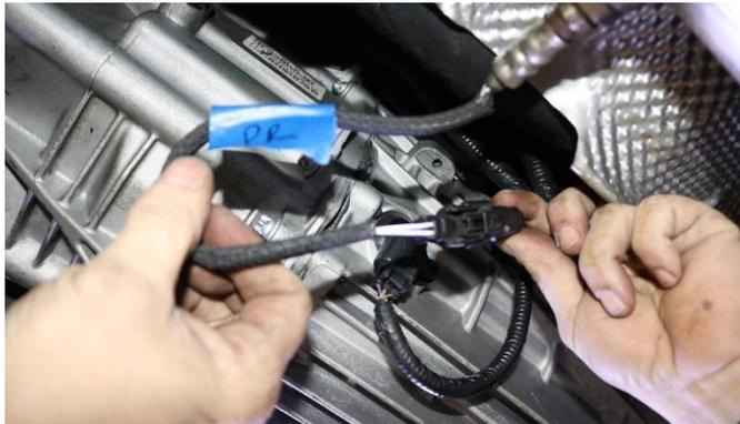
**7. WARNING:** Make sure you put the O2 sensors in the correct cat pipes as you marked them in the removal process.
