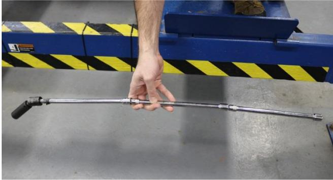
1. Locate the flange connecting the passenger catalytic converter to the manifold, from the top of vehicle in the engine bay remove the top nut nearest to the firewall using three 12" long 3/8" extensions, 3/8" swivel, and deep 15mm socket.
