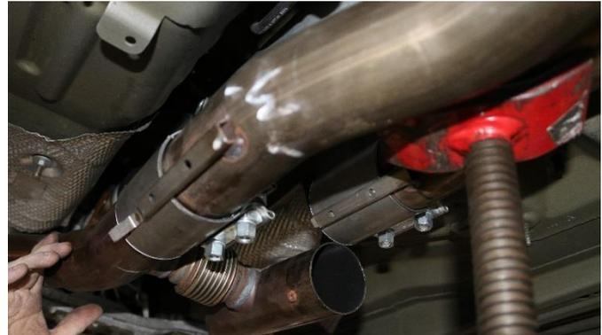
4. Support the factory axle pipes and the driver catalytic converter with a jack stand or similar device. **DO NOT let the exhaust droop as it may damage the rear bumper cutouts**
