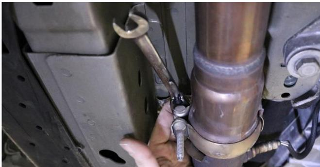
5. Loosen the spherical joint clamp on both the catalytic converters using a 13mm wrench.
