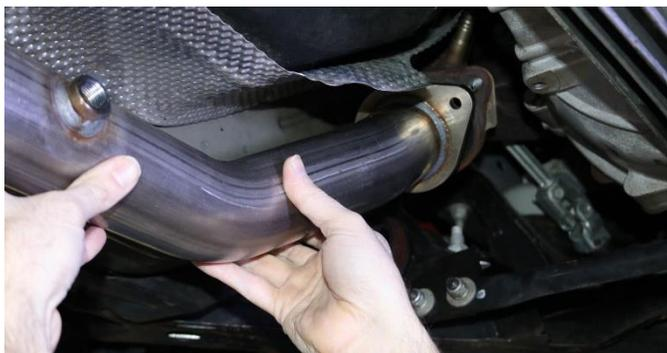
3. Place the off road pipe onto the bolts as shown.
