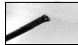
Bad cut - flattened
