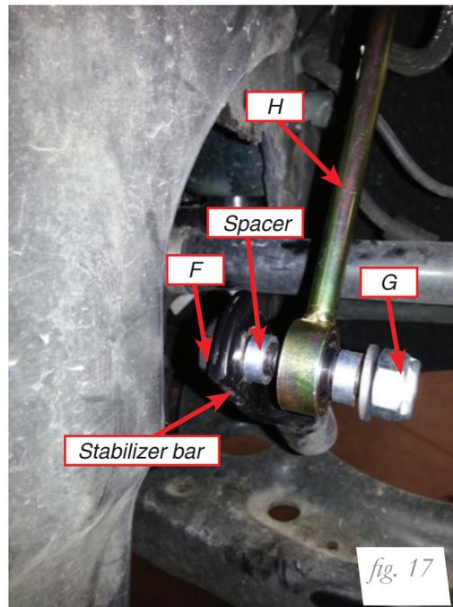
5. Attach the end link stud to the end link tab on the strut (fig. 18). Torque to 65 Nm (48 lb.-ft.).
