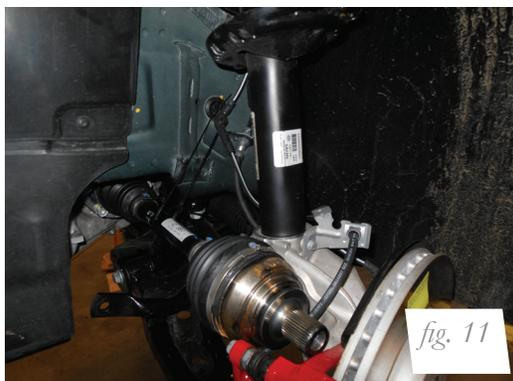
9. Unbolt the three upper strut mount bolts and remove the strut from the vehicle (figs. 12a and 12b).
