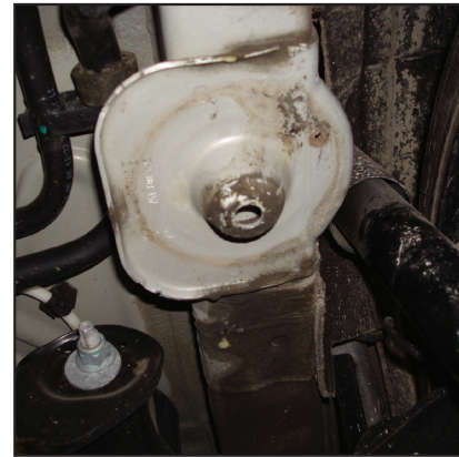
Previously Cut Spring Perch with Aftermarket Shock
