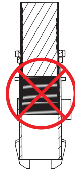
Not OK, threads are showing.
