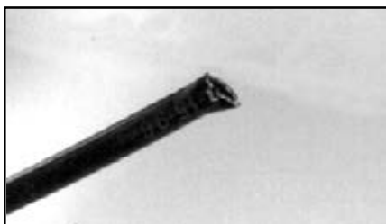
Bad cut - flattened
