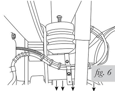
*Drop the axle slightly, if necessary, to position the jounce bumper between the frame and the axle.*
