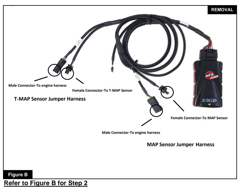
Step 2: Refer to the diagram to identify the connectors and their corresponding sensors that they plug into.
