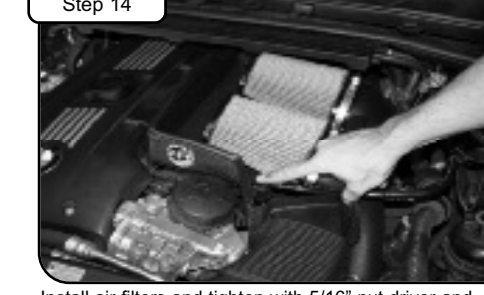
Step 14 Install air filters and tighten with 5/16" nut driver and connect vacuum line.
