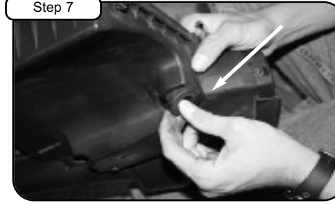
Step 7 Remove the 3 rubber grommets from the air box. (To be used in step 9.)
