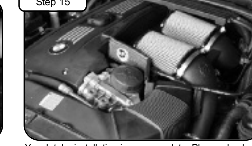
Step 15 Your Intake installation is now complete. Please check all clamps and hoses periodically and tighten.
