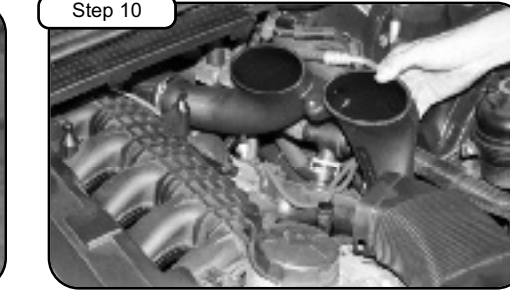
Step 10 Install new tube into vehicle and pull back towards driver fender. Do not tighten clamps.
