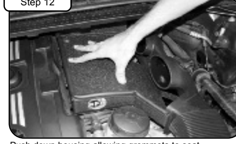
Step 12 Push down housing allowing grommets to seat. Align threaded insert with hole on housing.
