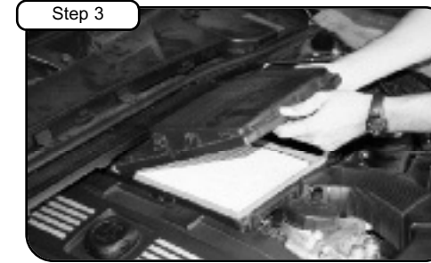
Step 3 Unclip upper half of air box to remove lid and filter.
