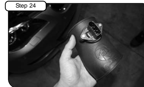
Step 24 Remove MAF sensor from airbox and install in new tube (05-00969) with screws and gasket provided. Tighten using flathead screwdriver.
