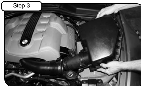
Unclip upper half of air box and lift carefully. Pull back MAF sensor from OE tube.
