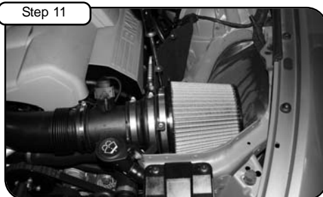
Install air filter and tighten using 5/16" nut driver. Re-connect MAF sensor harness.
