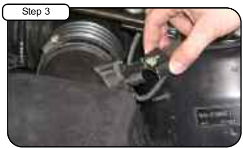
Step 3 Remove factory harness from MAF sensor and place out of the way until re-assembly.
