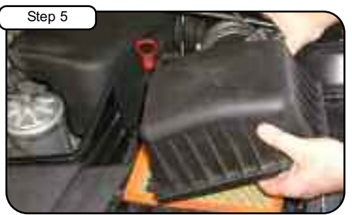
Step 5 Using a standard screwdriver loosen the clamp securing intake track to factory airbox. Undo clamps securing top half of airbox and remove top half. Set aside for future removal of stock MAF sensor.
