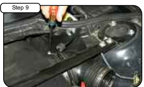
Step 9 Remove factory accordion coupler using 1/4" nut driver or flat screwdriver.
