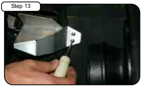
Step 13 Install Flow divertor onto housing using provided button head screws.
