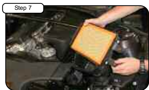
Step 7 Using a 10mm socket remove the remaining bolt holding the factory intake in place, remove the lower half of the intake. Set the bolt aside for re-installation of heat shield.
