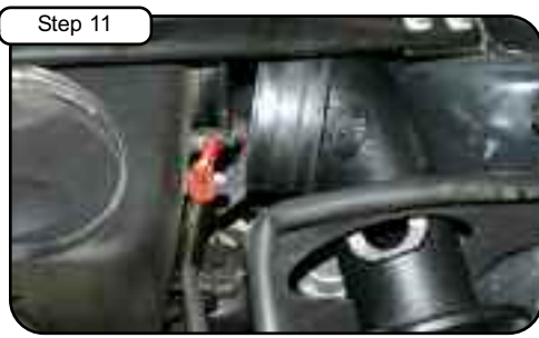
Step 11 Slide coupler onto tube and place tube through housing hole.
