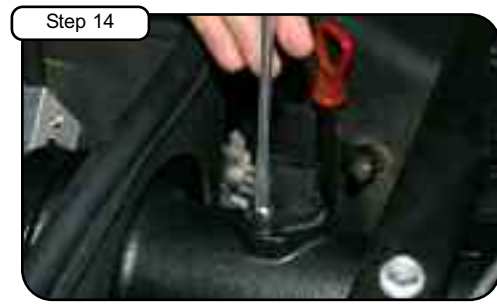
Step 14 Install MAF sensor onto tube using provided gaskets and screws.
