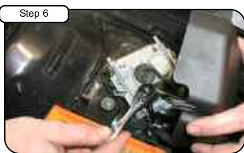
Step 6 Remove plastic cover from headlight controller via locking tabs. Using a 10mm socket, remove the (2) bolts securing controller to allow for its movement and to release lower half of airbox.
