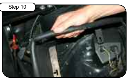
Step 10 Install trim seal on housing and drop housing into vehicle. Do not tighten down housing.
