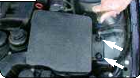
Remove two screws with 10 mm socket or wrench.
