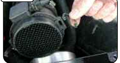
Attach supplied spring clips onto mass flow sensor insert hooked end into slotted section on mass flow sensor.
