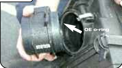
Remove the mass flow sensor from OE air box, and carefully pull out o-ring to save and re-use.
