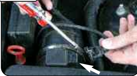
Remove mass flow sensor plug and hose clamp (1/4" nut driver)
