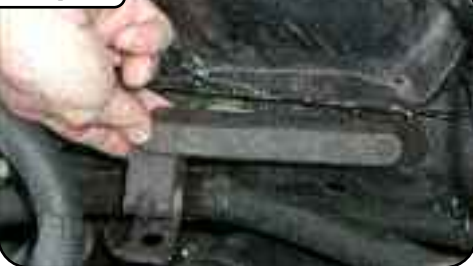
Remove rubber cushion at bottom of the fenderwell.
