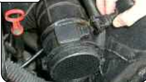
Install mass air flow sensor, tighten clamp with 1/4" nut driver and connect mass flow sensor plug.
