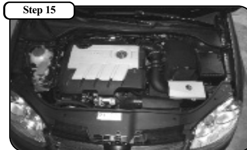
Your Stage 1 Intake is now complete. Make sure to tighten all clamps and check all electrical connections. Thank you for choosing aFePower! NOTE: Retighten all connections after approximately 100-200 miles.
