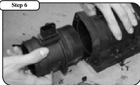
Using a phillips screwdriver, remove the MAF sensor from the stock cover.
