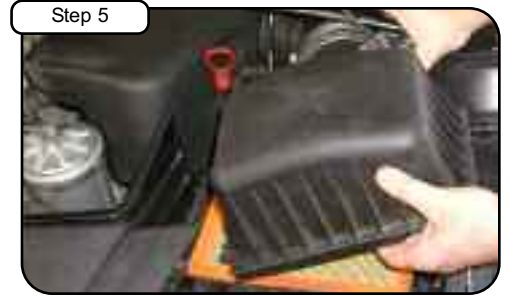
Using a standard screwdriver loosen the clamp securing intake track to factory airbox. Undo clamps securing top half of airbox and remove top half. Set aside for future removal of stock MAF sensor.
