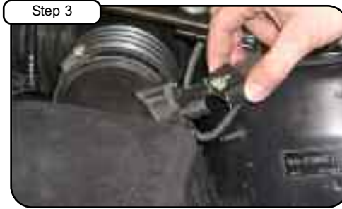
Remove factory harness from MAF sensor and place out of the way until re-assembly.
