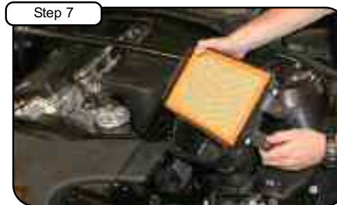
Using a 10mm socket remove the remaining bolt holding the factory intake in place, remove the lower half of the intake. Set the bolt aside for re-installation of heat shield.
