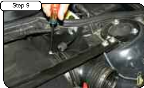
Remove factory accordion coupler using 1/4" nut driver or flat screwdriver.
