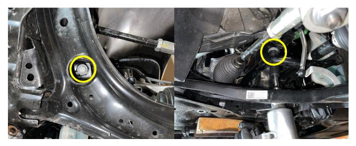
14F Lower the sub frame just enough so the sway bar can be removed towards the rear of the car. You will need to lift up to the steering rack and sneak the sway bar under and out the back.
