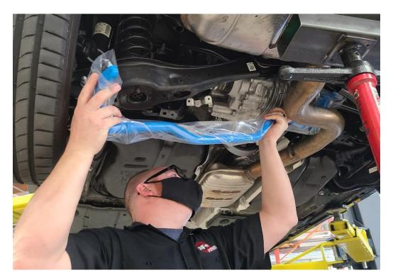
12R Grease the rear bushings with the supplied silicone lube.
