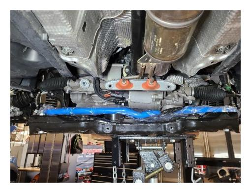
17F Grease the front bushings (5343) with the supplied silicone lube. Install bushing onto the sway bar. The bushings should be positioned just inside of the centering rings.
