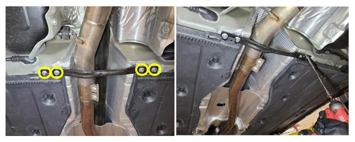
6R Remove center rubber hanger with a (13 mm socket).
