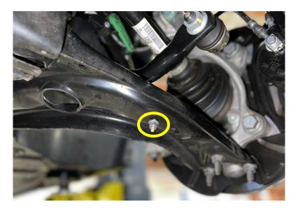
4F Disconnect the end links from the stock sway bar using a (18mm wrench) for the nut and (M6 Triple Square socket) for the stud.
