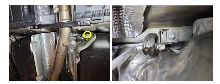
7R Disconnect the end links from the stock lower control arms using a (13mm socket) for the nut and (13mm wrench) for the stud.
