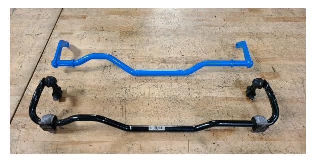
11R Install the rear aFe Control sway bar in the same manner as factory removal. We suggest leaving the sway bar in the poly bag when feeding it into the car. This will keep it safe from scratches. (remove poly bag once bar is in place)
