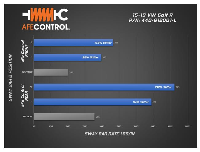
Stiffer roll resistance will demand more from the tires. When the tire's grip is overloaded, they will begin to slip. Manipulating when the front or rear tires slip can make the vehicle understeer, oversteer, or handle neutral. So, think of it as the higher the stiffness, the earlier the slip. If the front slips first, you will have understeer. If the rear slips first, you will have oversteer. If both front and rear slip near the same time, you will have neutral handling.
