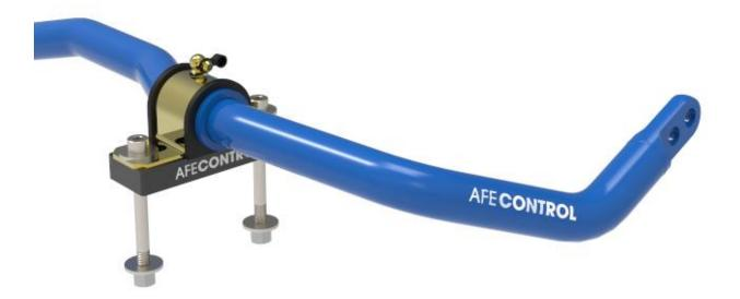
The bushing brackets are slotted to allow for positioning the bar. Make sure the bar has clearance between the steering rack and the subframe. Tighten the hardware to 29 ft  $\cdot$  lbs.
