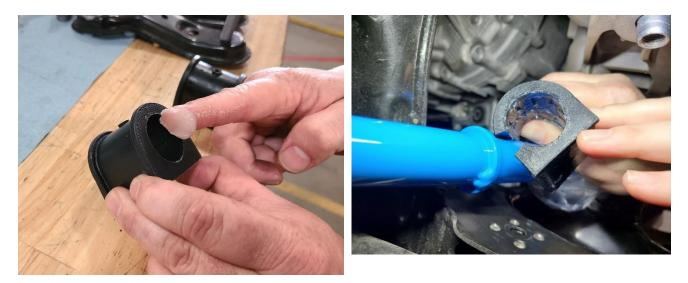
18F Slide the aFe Control bushing bracket onto the bushings and mate the sway bar assembly to the subframe. Use the supplied hardware kit (p/n 00P-0A1713-A) to secure the brackets to the subframe. See diagram below:
