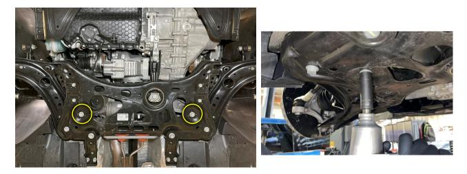
9F Unclip the oil sensor connector. Pry the push-clip to release sensor line from the subframe.
