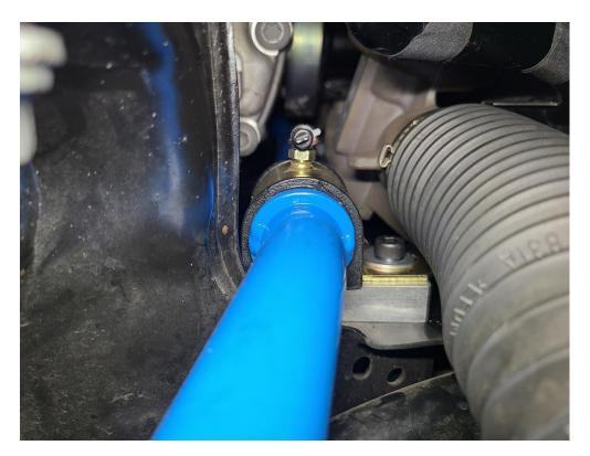
19F Perform steps 1F-14F in reverse order. When attaching the end links to the sway bar you have 2 settings: Medium and Stiff. The hole closest to the end is the Medium setting. Stiff Setting shown. (Tip: Apply medium thread locking compound on the end link stud to ensure the nut does not come loose)
