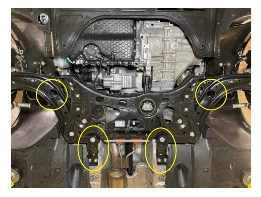
Undo the rear mount brackets with a (16mm and 18mm sockets).
