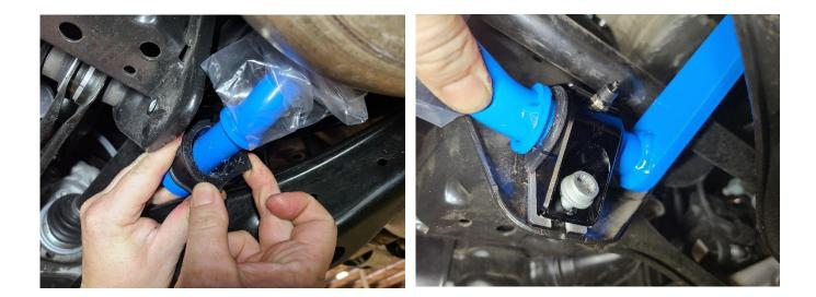
14R Make sure the provided end link is correctly assembled. And adjusted to the shortest length. Install the provided end link onto the sway bar, then mount the end link to the subframe with a (17mm wrench and a 15mm socket). Tighten to **35ft Ibs**. Do not use an impact gun or over tighten.
