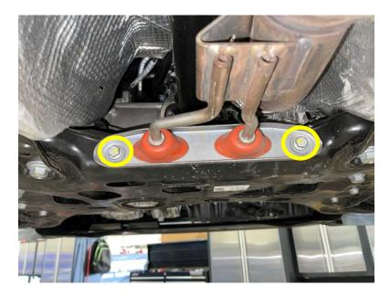
6F Disconnect the dog bone mount with a 18mm wrench and socket.
