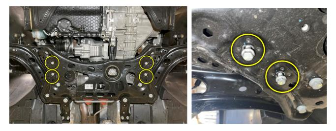
8F Undo the (2) steering rack bolts with a (18mm socket).
