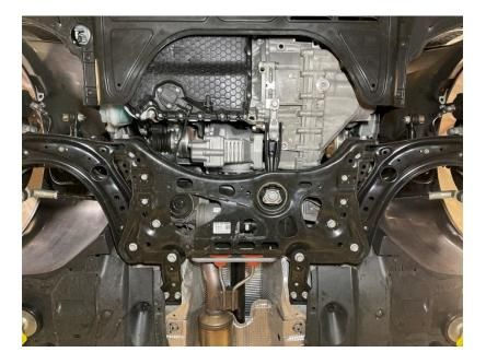
3F Disconnect the ride height sensor from the driver side lower control arm, using a 10mm socket.
