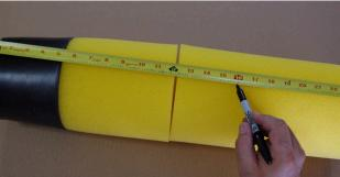
3. Using a bread knife or hacksaw with fine-tooth blade, carefully cut the additional foam section to the desired length.
