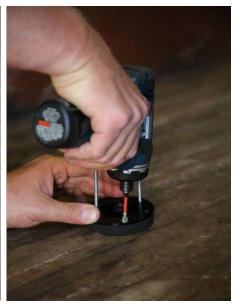
8. Once four of the screws are started, remove the two studs and insert the two remaining screws in the holes. Now fully tighten the filler cap screws, they just need to be tight enough to compress the gasket and sit flush against the mounting surface. Do not overtighten the screws to avoid damaging the housing.
