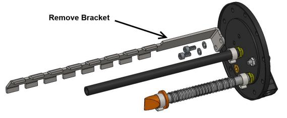
5. Remove the original fuel supply line from the standard Phantom fuel pump hanger assembly. To remove the original pinch clamp from the line, grasp the pinched portion of the clamp with a pair of pliers and twist to loosen.
