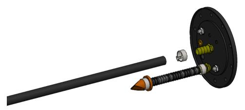
8. Using the 5/32" Allen wrench, install the longer fuel pump bracket from the extension kit. If you have lost any of the original hardware, don't worry, replacement hardware is included in your extension kit.
