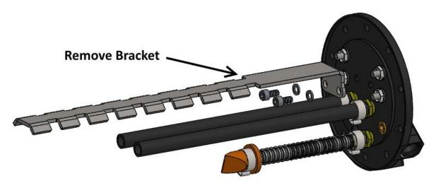
5. Remove each of the original fuel supply lines from the standard Phantom fuel pump hanger assembly. To remove the original pinch clamps from the line, grasp the pinched portion of each clamp with a pair of pliers and twist to loosen.
