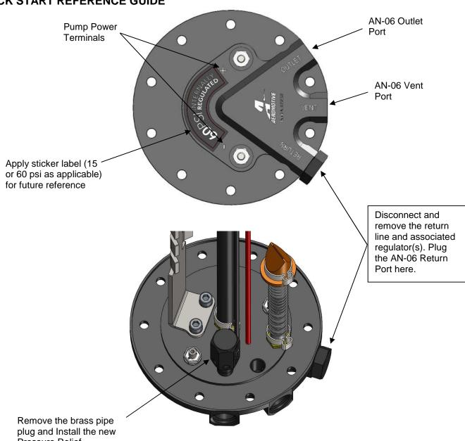
Pressure Relief (Bypass) Valve here If this has not been done already, we <u>strongly recommend</u> installing a remote-mount rollover valve. It must be mounted in a vertical position and mounted as high or higher than your filler tube.
