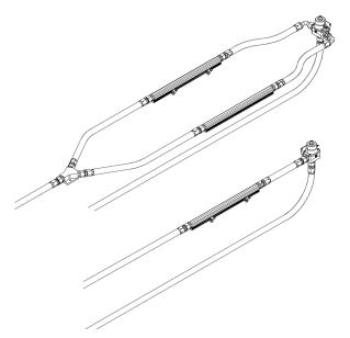
5. If you are running a Carbureted System, connect the fuel filter outlet to a Bypass style fuel pressure regulator (Aeromotive p/n 13204 or similar).
