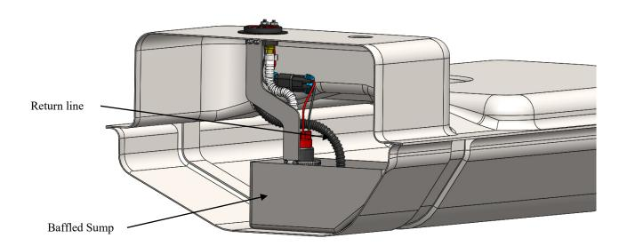
9. Install either ORB-06 x AN flare 90-deg fittings with the AN male sized to match your fuel lines (for AN-06 line use Aeromotive PN 15689; for AN-08 line use Fragola PN 499207BL, or other like fittings).
