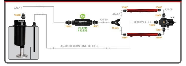
5. If you are running a Carbureted System, connect the fuel filter outlet to a bypass style fuel pressure regulator and/or fuel log as in the following diagrams.
