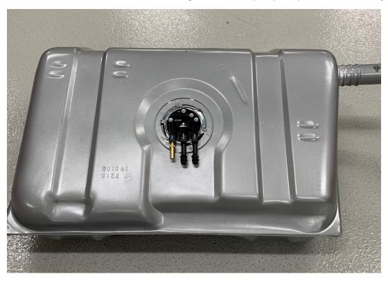
8. Connect the supply and return fuel lines to the new Aeromotive fuel pump assembly. The supply and return fittings are AN-06 male flare and will require AN-06 female hose ends. The vent port is a 3/8" hose barb in which the OEM vent hose can reattach to. Note: AN-08 lines will be required for carbureted applications; AN-06 or AN-08 lines may be used for EFI applications.
