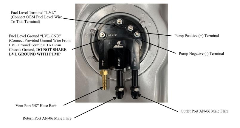
9. Connect power to the fuel pump terminals as shown in the following diagram.
