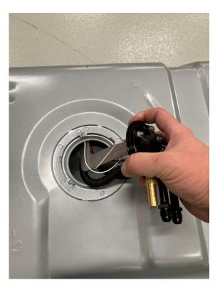
7. Ensure that the fuel pump locking ring gasket is still positioned properly in the receiver groove and then install the locking ring. Note the orientation of the outlet cap fittings in the following image, the fittings need to point towards the front of the tank to ensure the sending unit arm and pump are positioned correctly in the tank.
